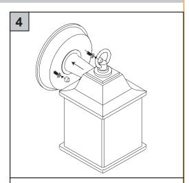
Place the silicone washe remove in Step 1 onto the screw, then fully secure the fixture by han-tightening the nut.
