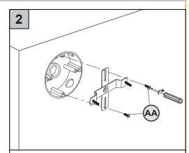
Attach the cross plate to the junction box with part AA.
