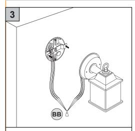
Using part BB, connect the fixture wires to the junction box wires. Then carefully insert the wires into the junction box.
