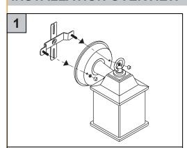
Take out part A from the package, unscrew the nut by hand, an remove the nut, silicone washer, an cross plate.
