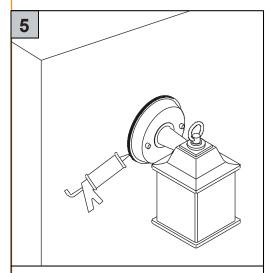
Use a glue gun to apply a bea of sealant aroun the base. Installation is complete.
