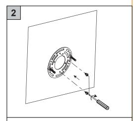
Secure the Bagua plate to the mounting box.
