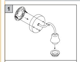
Remove part A, unscrew the hand-tightened nut on the light fixture, take off the Oring silicone gasket, then unscrew and set aside the outer ring from the E26 lamp holder.
