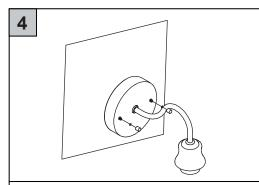
Place the light fixture onto the screws of the Bagua plate, then slide on the silicone gasket and tighten the hand-tightened nut.
