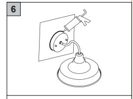
Apply sealant for watertight protection.
