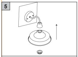
Insert part B into part A, then use the outer ring removed in step one to screw and secure B onto A.
