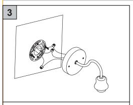
Connect the corresponding wires properly.
